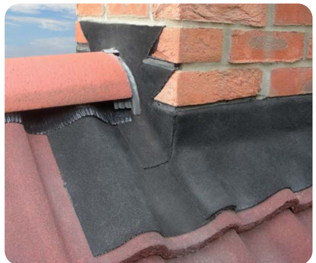
Photograph taken at BRE immediately after 49m/s (110mph) wind tunnel test
